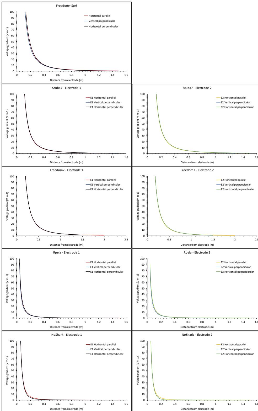
**Figure 7.** Modelled voltage gradients of the electric fields emitted by the shark deterrents measured in this study. Each curve was obtained by finding the least-squares best fit of the standard electrostatic field equation to electrical potentials measured at different distances from each electrode. Distance zero is equivalent to the centre of one electrode of the device. Both electrodes in the Freedom+ Surf had the same emission characteristics.
