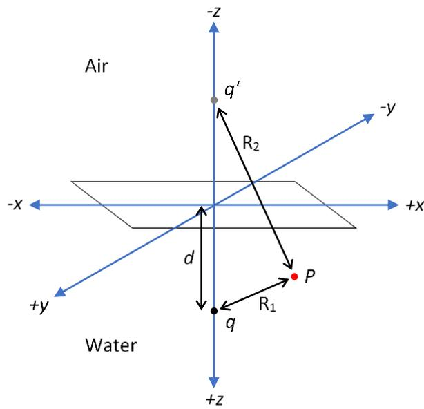
**Figure 2.** Geometry for modelling the electrical potential generated by a single electrode of a repellent device in a dielectric half space. The horizontal  $(x, y)$  plane at  $z = 0$  represents the air-sea interface.  $q$  is the charge on the electrode;  $q'$  is the mirror charge;  $d$  is the distance of the electrode from the surface;  $P$  is the location of the voltage measurement.
