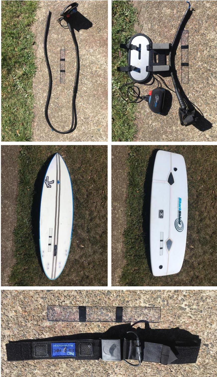
**Figure 1.** Photographs of the electrical deterrent devices measured in this study. Clockwise from top-left: Freedom 7, SCUBA7, Freedom+ Surf, NoShark and Rpela. The size indicator in each image is a 30 cm ruler with black tape indicating a 10 cm distance.
