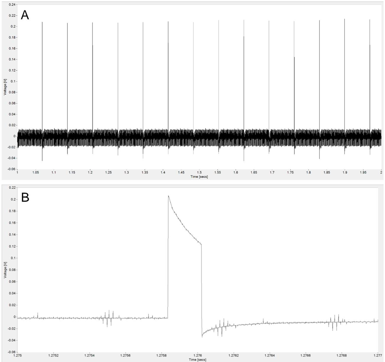
**Figure 5.** Emitted electrical pulse waveforms for the Rpela. (A) Sequence of pulses showing fixed polarity from a single electrode with a pulse frequency of  $\sim 14.5$  Hz; (B) A single positive-going pulse of  $\sim 0.2$  ms duration.
