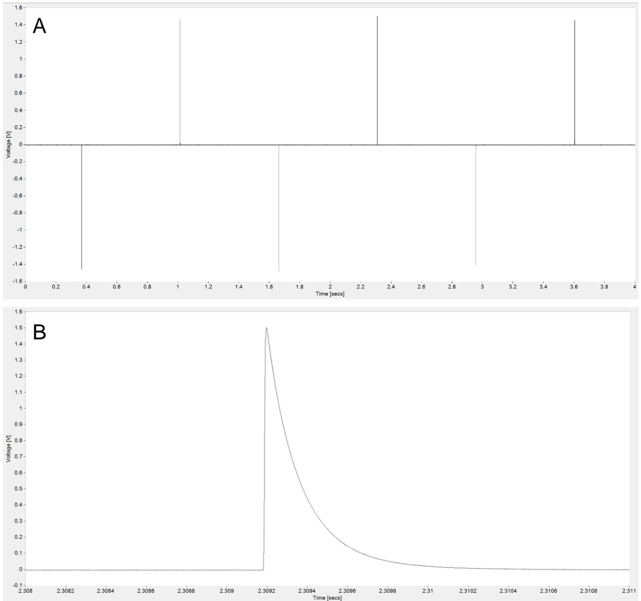
**Figure 4.** Emitted electrical pulse waveforms for the Shark Shield Freedom 7. (A) Sequence of pulses showing alternating polarity from a single electrode with a pulse frequency of  $\sim 1.5$  Hz; (B) A single positive-going pulse of  $\sim 1$  ms duration.
