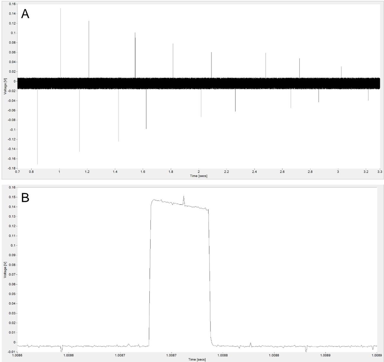
**Figure 6.** Emitted electrical pulse waveforms for the NoShark. (A) Sequence of pulses showing fixed polarity from a single electrode with a pulse frequency of ~7 Hz; (B) A single positive-going pulse of ~0.1 ms duration.
